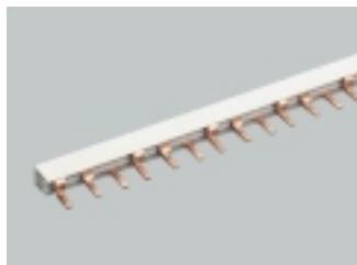
31102 comb type busbar, insulated, 3-pole, bridge type 65 A, pitch 27 mm, 1 m long
